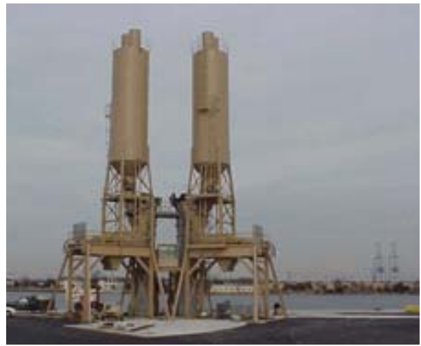
Gravity feed dual pugmill system
