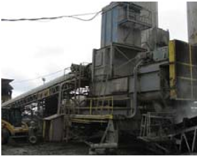
Conveyor feed single pugmill system
