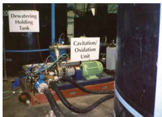
BioGenesis™ oxidant injection
