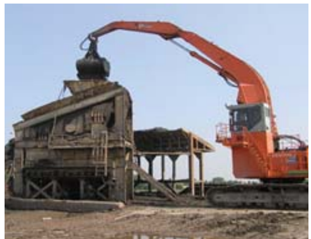
Gravity feed dual pugmill system
