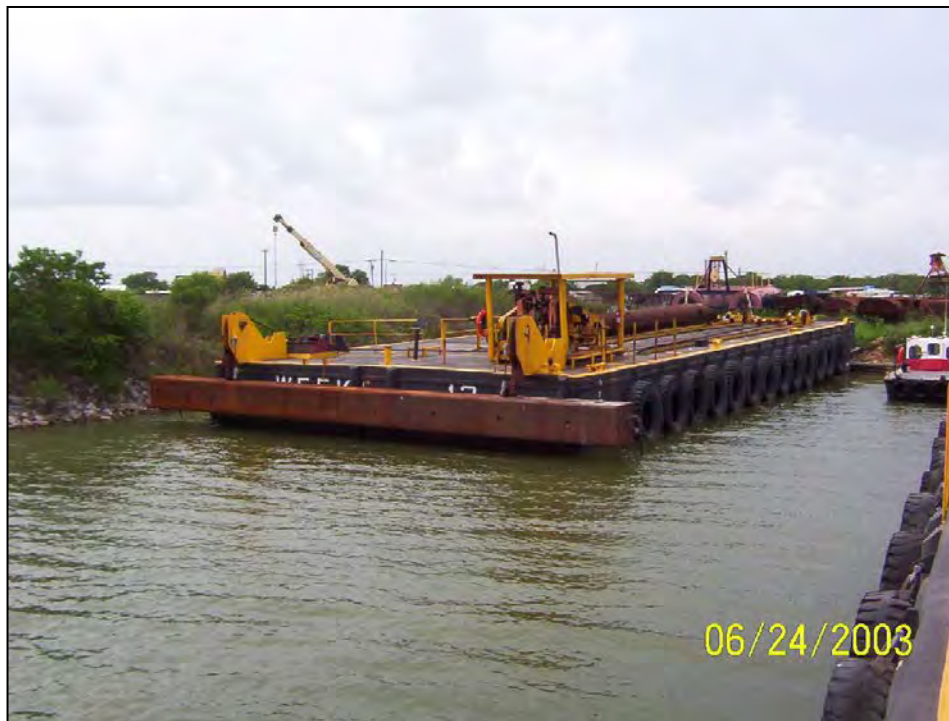
Figure 2-40. Bed-Leveler Suspended from a Work Barge (Photo Courtesy of Weeks Marine, Inc., Cranford, NJ)
