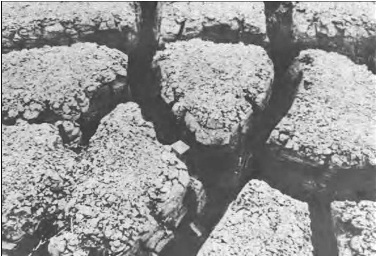
Figure 4-36. Desiccation Crust Achieved in Highly Plastic Clay Dredged Material 180 m (200 yd) into a Placement Area by Perimeter Trenching over a 12-month Period
