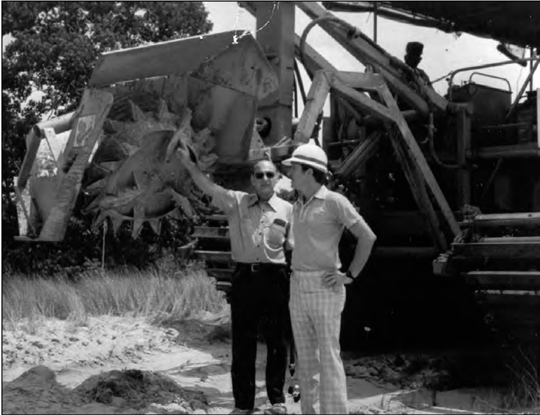
Figure 4-39. Hemispherical Rotary Trenching Implement
