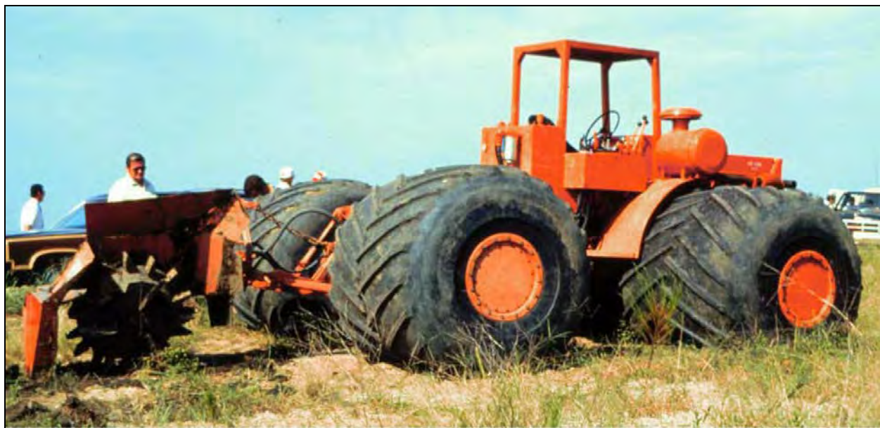
Figure 4-37. Rubber-Tired Rotary Trencher
