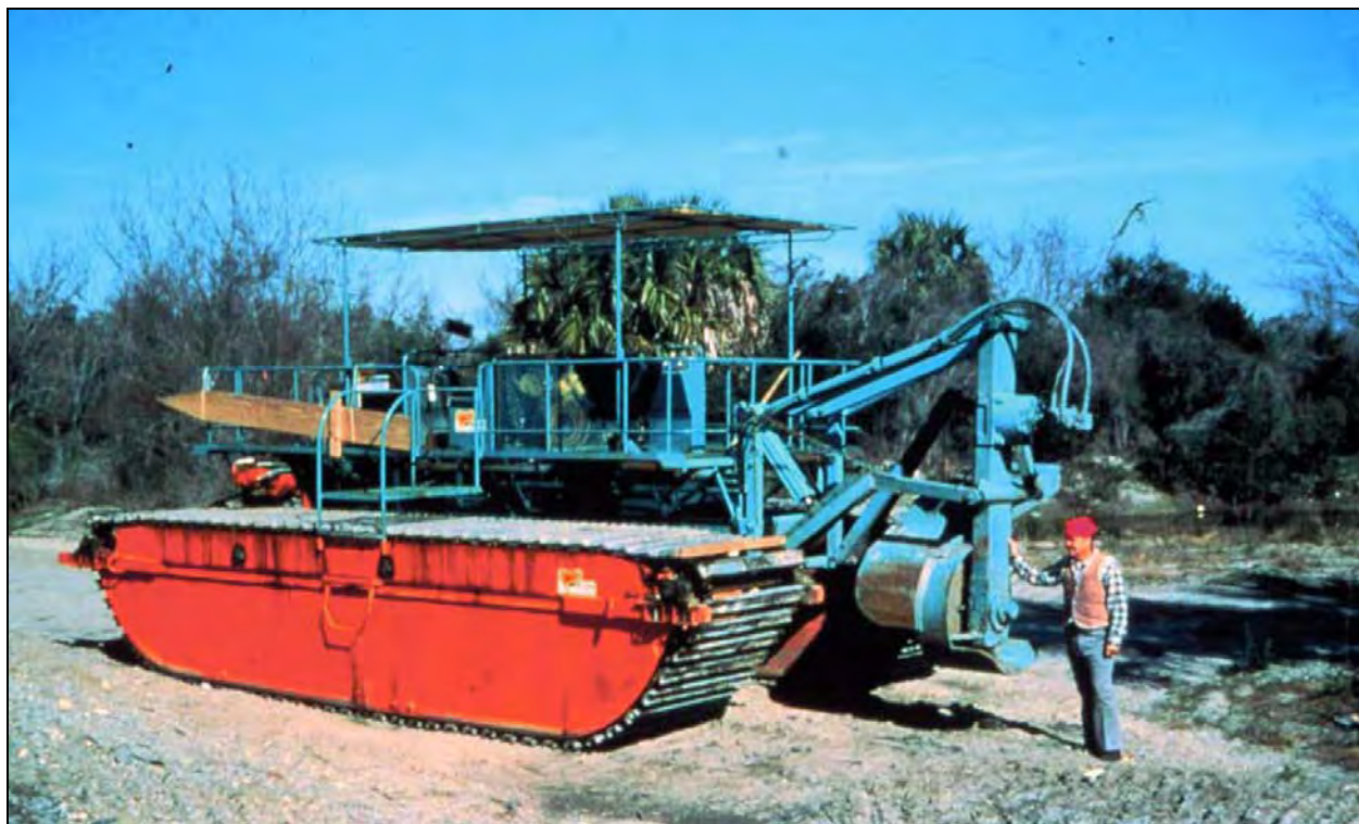
Figure 4-38. Track-Mounted Rotary Trencher Used in Mosquito-Control Activities
