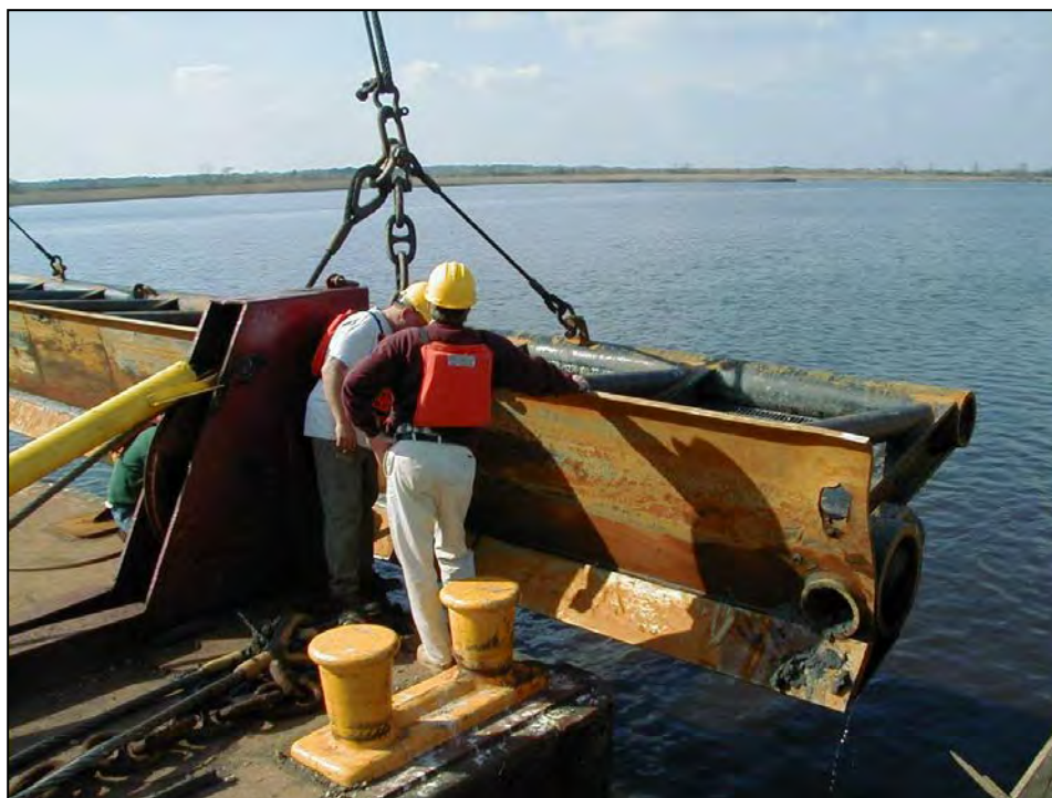
Figure 2-41. Bed-Leveler Suspended by an A-Frame on a Work Barge (Photo Courtesy of Great Lakes Dredge and Dock Company)
