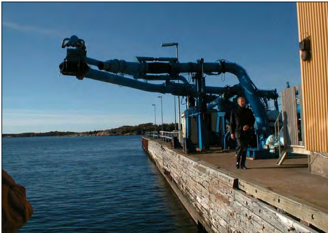
Figure 4-8. Specialized Hydraulic Offloaders
