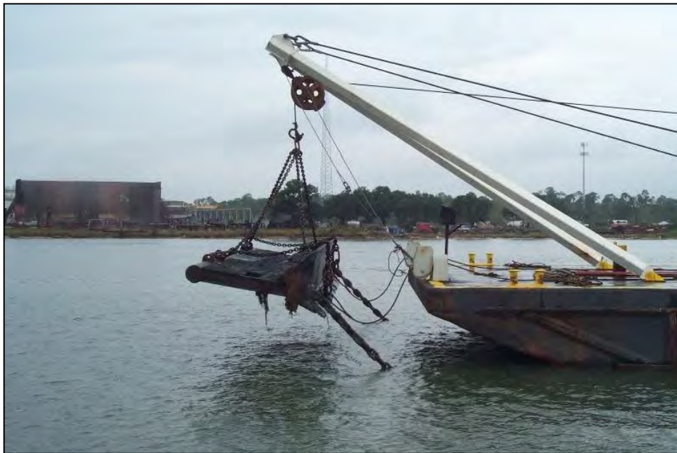
Figure 2-39. Bed-Leveler Suspended by an A-Frame on a Work Barge (Photo Courtesy of Bean Dredging Company, New Orleans, LA)
