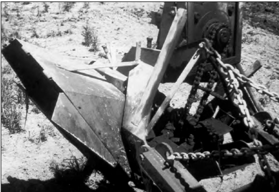
Figure 4-40. Trapezoidal Rotary Trenching Implement
