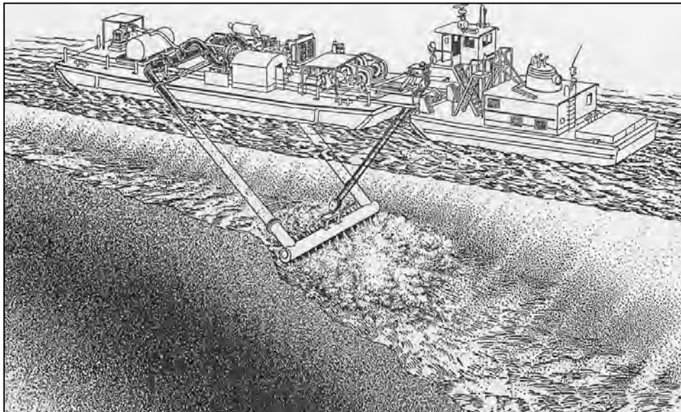
Figure 2-38. Water Injection Dredge
